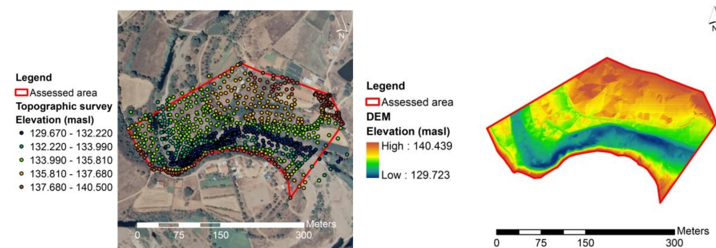
Fig. 4. Points of the topographic survey in the Portuguese site (left) and Digital Elevation Model obtained with the ESRI® ArcGIS™ 9.2 software (right).
